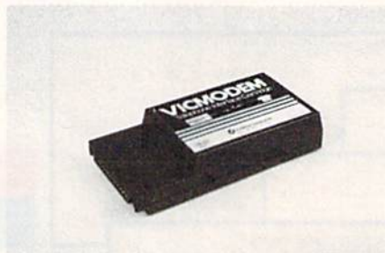
The VICmodem is an example of a direct-connect modem - it bypasses the telephone handset.
